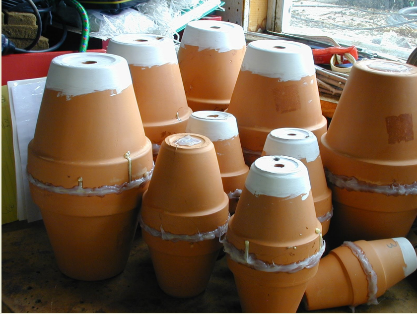
Ollas made at home using caulking, clay pots and a rubber stopper
