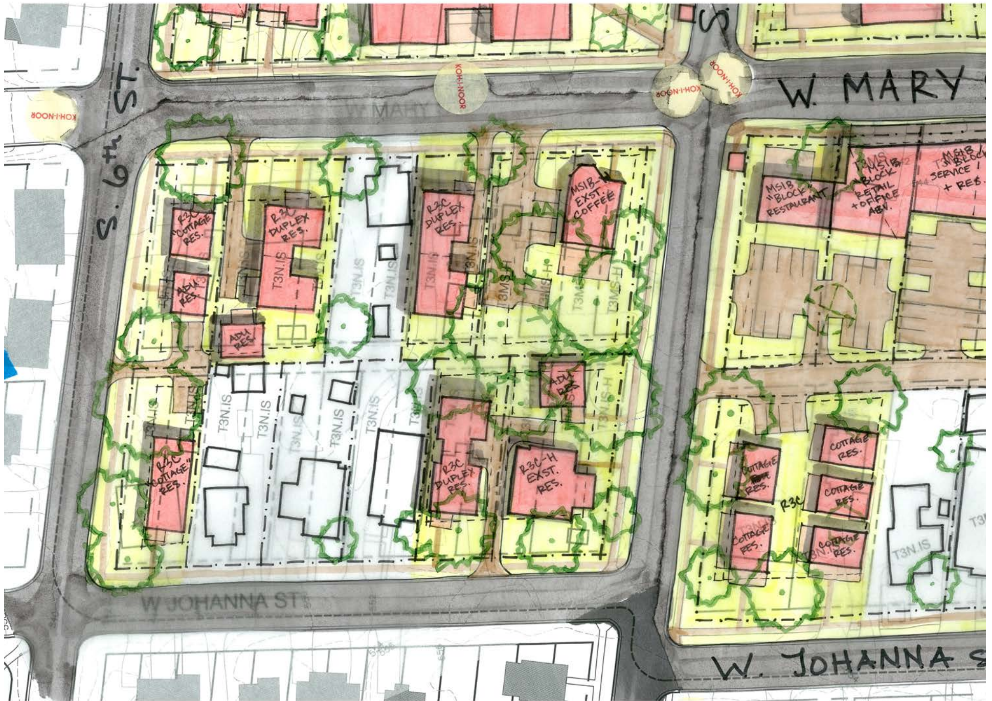
Figure 2.4: R3C development without an alley
