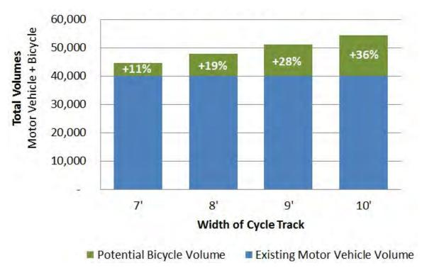
ADDITIONAL CORRIDOR VEHICLE CAPACITY ON SOUTH LAMAR WITH ADDED CYCLE TRACKS OF VARYING WIDTHS. SOURCE: CITY OF AUSTIN.
