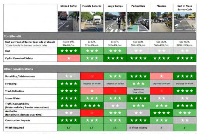
EXCERPT OF CHART SHOWING FACTORS REQUIRING SPECIAL CONSIDERATION WHEN SELECTING THE APPROACH FOR A PHYSICAL BARRIER. SOURCE: CITY OF AUSTIN.
